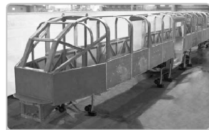
Prototype Colorado Railcar DMU under construction — a fine example of 1950’s-era design methods.
