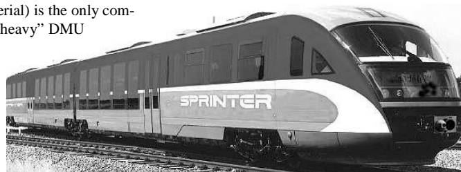
A DMU is a train type that does away with the locomotive. The Siemens Sprinter “light” DMU (shown above) has an extensive service record in Europe, and will soon be put to use in San Diego county. SMART refused to even study “light” DMU’s in its EIR. Other agencies using “light” DMU’s include New Jersey Transit and (probably) BART for the eBART extension to Antioch.
