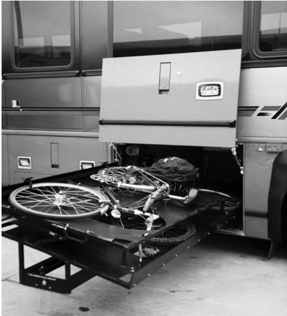
Prototype bus luggage-bay rack that holds two bikes. By using a front rack and racks in two luggage bays, AC Transit is working with Sportworks Racks to augment the bicycle capacity on each of their new 45-foot transbay and express buses to six bikes.
