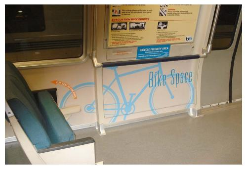
Bungee-ready "Bike Space" retrofit of 80 BART cars will each allow up to four bikes to be stacked against a leaning bar next to the door. Seen above is an early prototype equipped with a folding seat that compromises the Bike Space. The problematic folding seats will not be added to the remaining cars to be retrofitted using Safe Routes to Transit funds.
