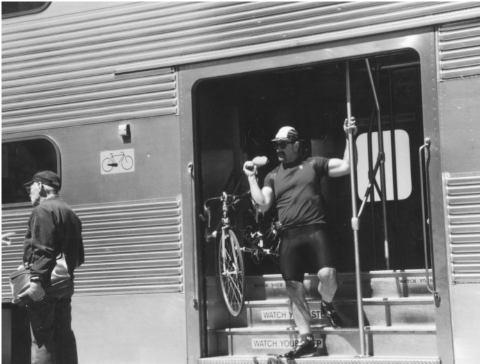
Steep stairs on Caltrain's Gallery car. Purchased in 1998, these cars have poor accessibility, which greatly increases station dwell time.
