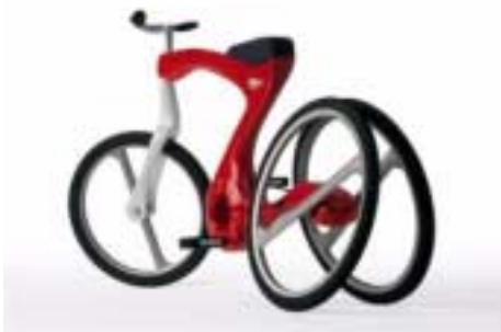
The advanced bicycle design pictured above comes from Dr. Scott S. Shim at Purdue University. It was created to make it easier for kids to learn how to ride a bike. "The 16-inch-wheel bicycle looks like a tricycle, but as the child gains momentum and learns to balance, the two rear wheels shift inward to merge into one wheel. This causes the balance to gradually shift from the bicycle to the child."
