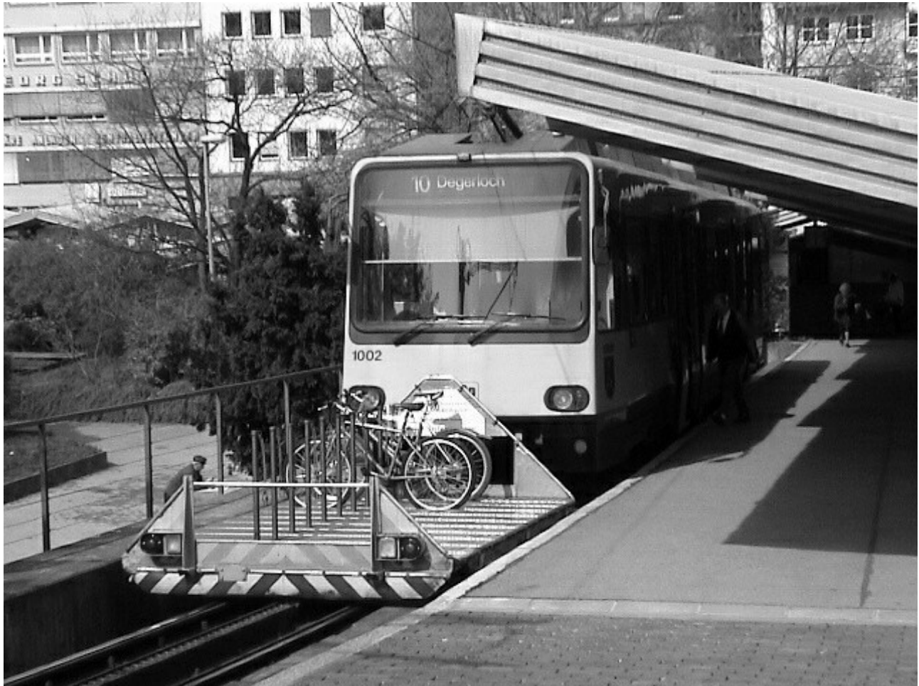
A special line in the Stuttgart (Germany) rail network is Line #10, a rack railway between Marienplatz and Degerloch stations. This train has a special bicycle car so bikers don't have to climb up the steep hill. ( www.metropla.net )
